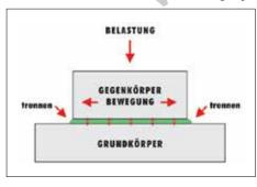
Despite a high pressure load and the shearing movement of the base body, the lubricating film of the HHS 2000 remains active and does not pull away. Reliably separates counter body from main body, thus ensuring optimum wear protection under high pressure loads. This is only possible with dirt-free lubricating points, which is why we recommend careful and thorough pre-cleaning with HHS Clean, Art. 0893 106 10, before each use.
